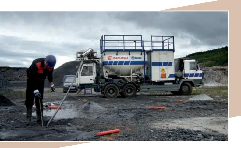
The EMSIT® V opencast explosive EMSIT® 20 is an explosive of a modern emulsion type with a high detonation velocity and outstanding resistance to water. The explosive is packaged by a modern cartridge machine into a thermally and mechanically resistant foil with a high strength weld.
